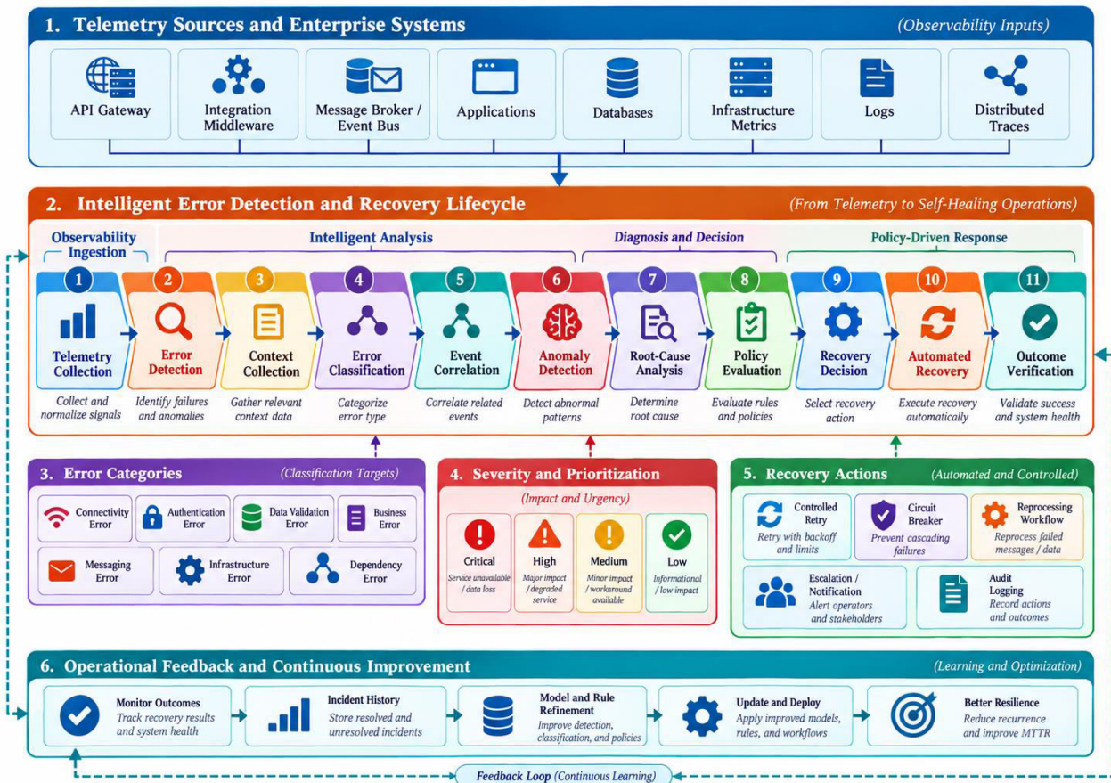
Fig. 2. Intelligent Error Detection, Classification, and Automated Recovery Lifecycle.
